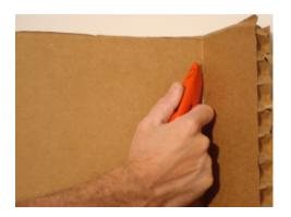
Using the safety utility knife included in your kit, cut into the surface of the panel, "snap" the panel, then turn the panel over to finish the cut on the back side.
