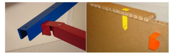
Throughout construction, use connectors at both the top and bottom of the panels, securing with twist nails at the top.
