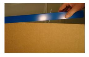
To remove the connector from the panel, simply lift the end and remove the nails.
